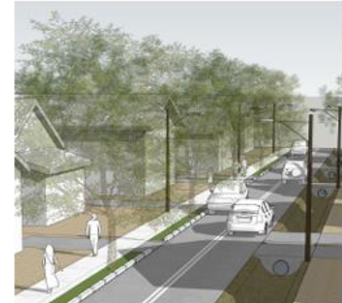
OD-3.3 Rendering of open ditch converted to a standard underground drainage system with a sidewalk and planting strip on top
