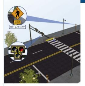
A Pedestrian Hybrid Beacon head consis lenses above a single yellow lens. Unlike the PHB rests in dark until a pedestrian a pushbutton or other form of detection. W the beacon displays a sequence of flash lights that indicate the pedestrian walk in is safe for drivers to proceed (see figure (
